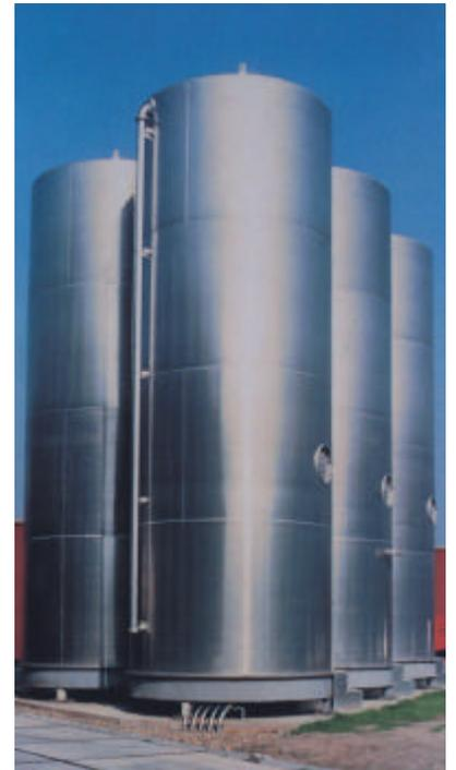
Accepted loadings for standard silo design: + 45/-5 mbar
